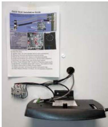
Photo: Correct routing of cables to avoid radio interference with base antennae.
